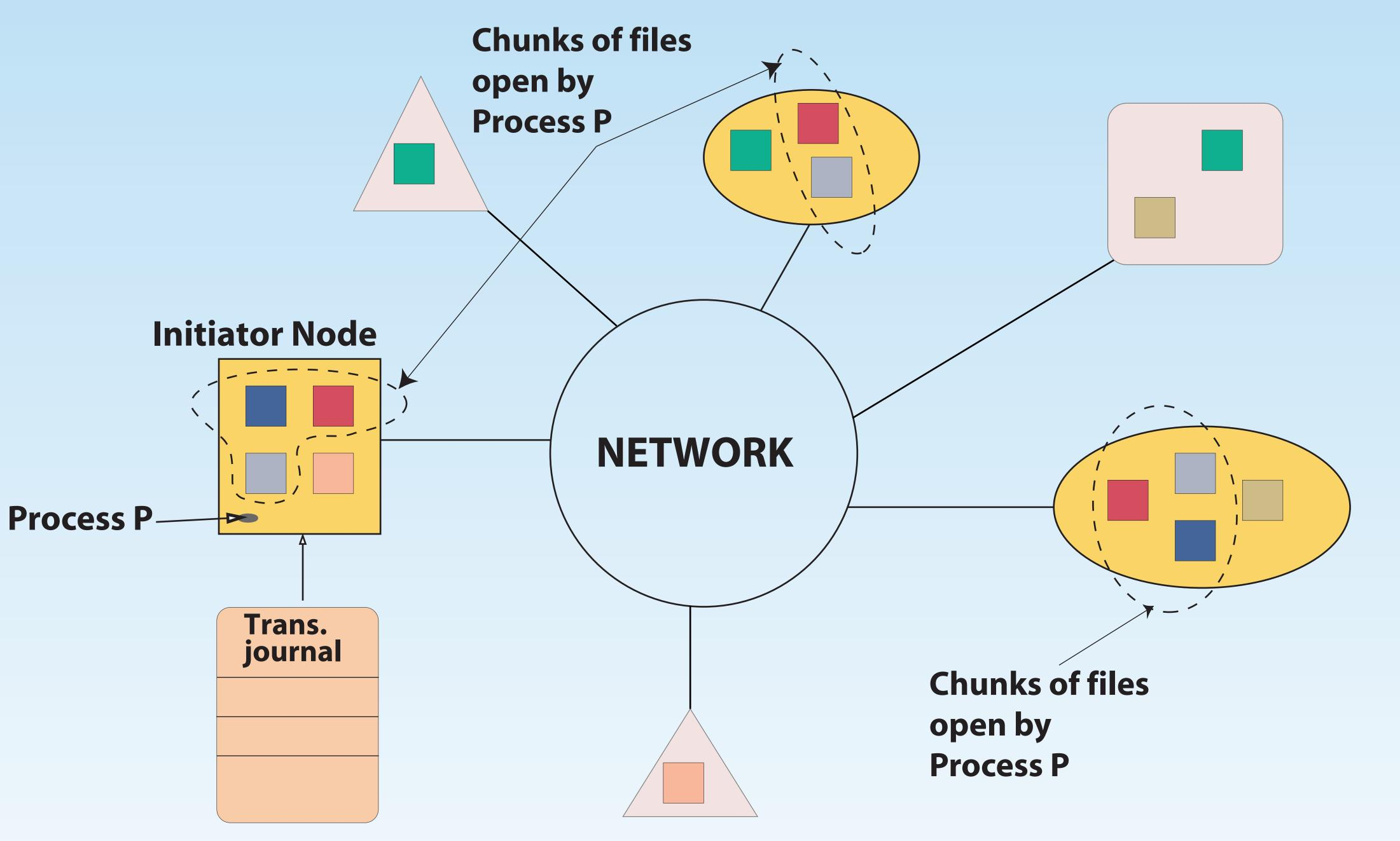
into smaller "chunks" which increases data availability and decreases the access time. It also makes it easier to replicate data across the system.
